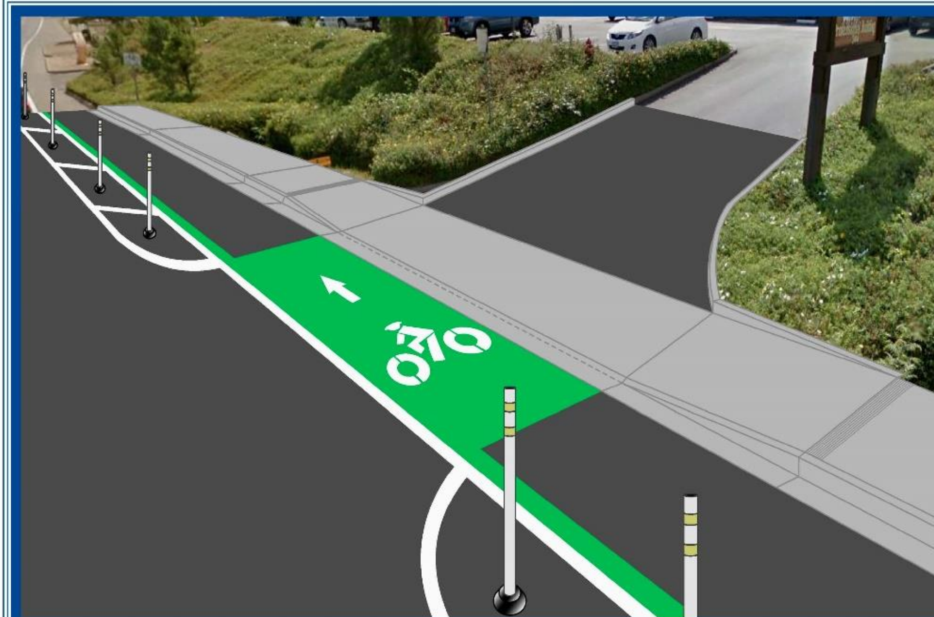
Rendering of Class IV Bike Lane "Cycle Track" to replace existing substandard Class II Bike Lanes
